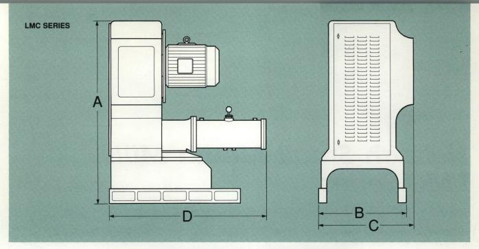
The LMC Molinex systems are designed to operate in low to medium viscosities. Applications with solids up to 75% in some systems are possible. The LMC John systems are also capable of processing ultrahigh viscosities (up to 750,000 cps) and high solids (up to 85%).
